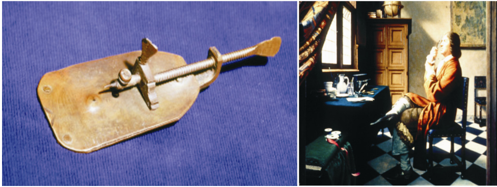
Figure 1: Original Antonie van Leeuwenhoek Microscope property of the Utrecht University museum, the Netherlands. The instrument consists of two brass plates (2.4x4.6 cm) riveted together at 3 locations. The hole contains a lens. On the tip of the sharp pin an object can be placed for observation. By using the screw on the pin one is able to focus the image. Van Leeuwenhoek made about 500 microscopes of which 9 have survived. This Utrecht example has a magnification of 266 X, while the other remaining magnify between 70 until 170 X. The Utrecht microscope allows for the observation of samples with a size of 0,00135 mm. Only after 1840 AD it was possible to build microscopes which could be used to study smaller objects. Antonie van Leeuwenhoek was not the original inventor of the microscope. Around 1600 a spectacles maker from Middelburg in the Netherlands found out that smaller objects could be more easily observed when placing two lenses at certain distance from each other. The microscope shown here was discovered around 1850 in the physics laboratory at the Minrebroederstraat in Utrecht the Netherlands by Prof. P. Harting. It was kept in a leather lined box with the inscriptions BB. Focal point 0,94 mm, Magnification 266x, Lens aperture 0,7 mm, Resolving power 1,35 mm. The painting showing van Leeuwenhoek using his microscope is by Robert A. Thom and appeared in "Great Moments in Medicine" published by Parke Davis & Company, in 1966.
